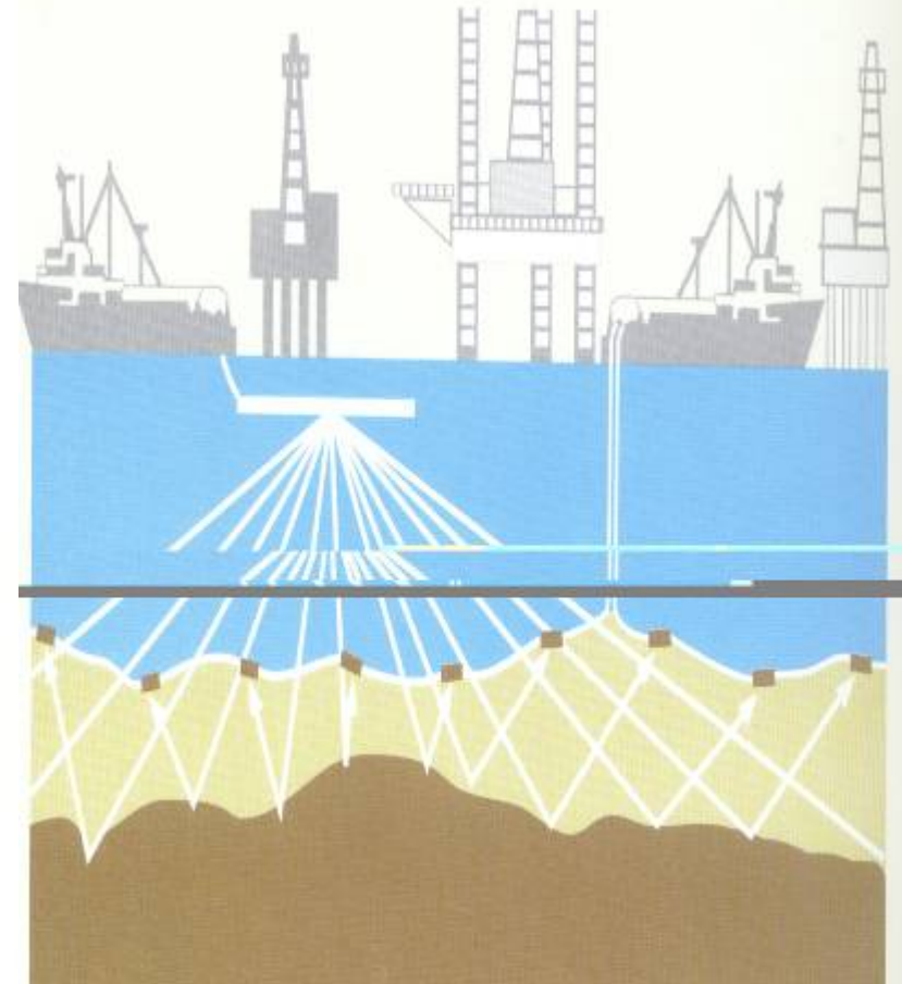
Figure 2.31. Schematic diagram of a marine seismic profiling system. (Modified from McQuillin et al., 1979.)
